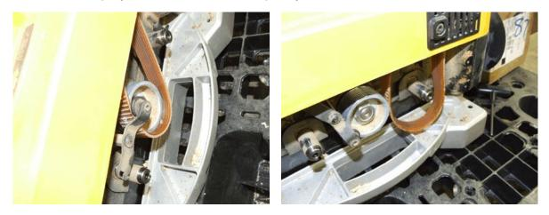
11. Remove the nut and washer from the end of the head.
