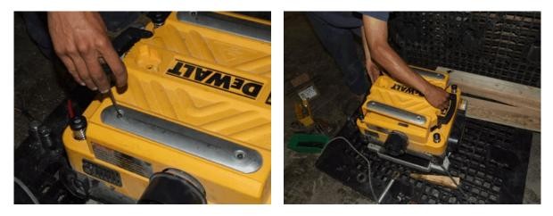
2.Remove the 3 red thumb screws from the inside of the top, then remove the inside dust cover. Doing this will expose the cutterhead.
