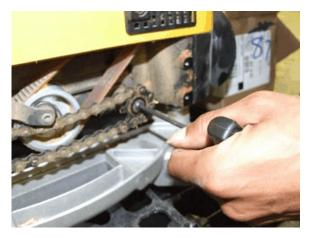
9. Remove the chain and sprockets together.
