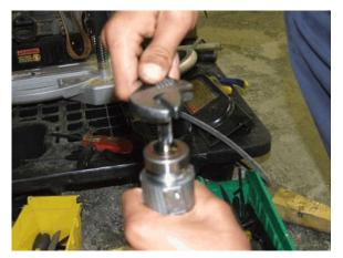
23. Install the bearings on each end of the new SHELIX(r). Install the key and screw the helical gear onto the end of the head.
