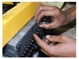
17. Remove the chain and sprockets together.
