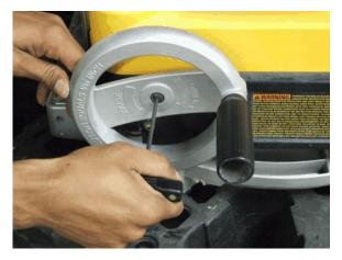
6. Remove the 4 screws and cover. This will expose the feed chain and pulley.
