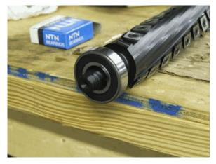
24. Carefully slide the new head through the bearing housing. Be careful of alignment so as not to bind the carbide knives and chip or break them.
