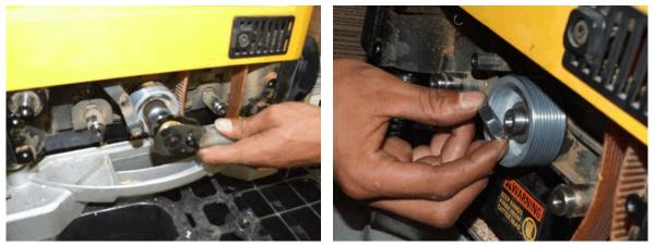
12. Slide the pulley off taking care not to lose the key.
