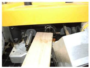
22. After the head is removed by sliding it through the bearing housing, unscrew the helical gear from the end of the head.
