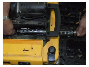
25. Carefully tap the head into position making sure the bearings are fully seated in the housings.
