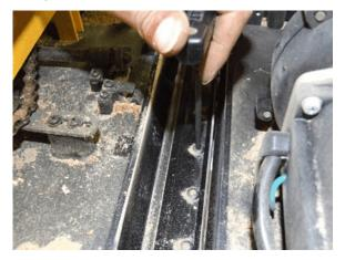
4. Remove the cutter rotate lock plate by removing the two phillips head screws. Be careful to catch the spring that is underneath the bracket.
