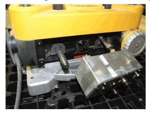
21. From the side opposite of where the pulley was, tap the head out using a piece of hardwood.
